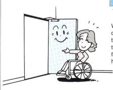
With this function, the door can be holdopened 2 — 10 seconds (adjustable) and then closes normally. This delayed-closing time, operative between 85° and 180°, facilitate passage by physically handicapped people, wheelchairs etc.
